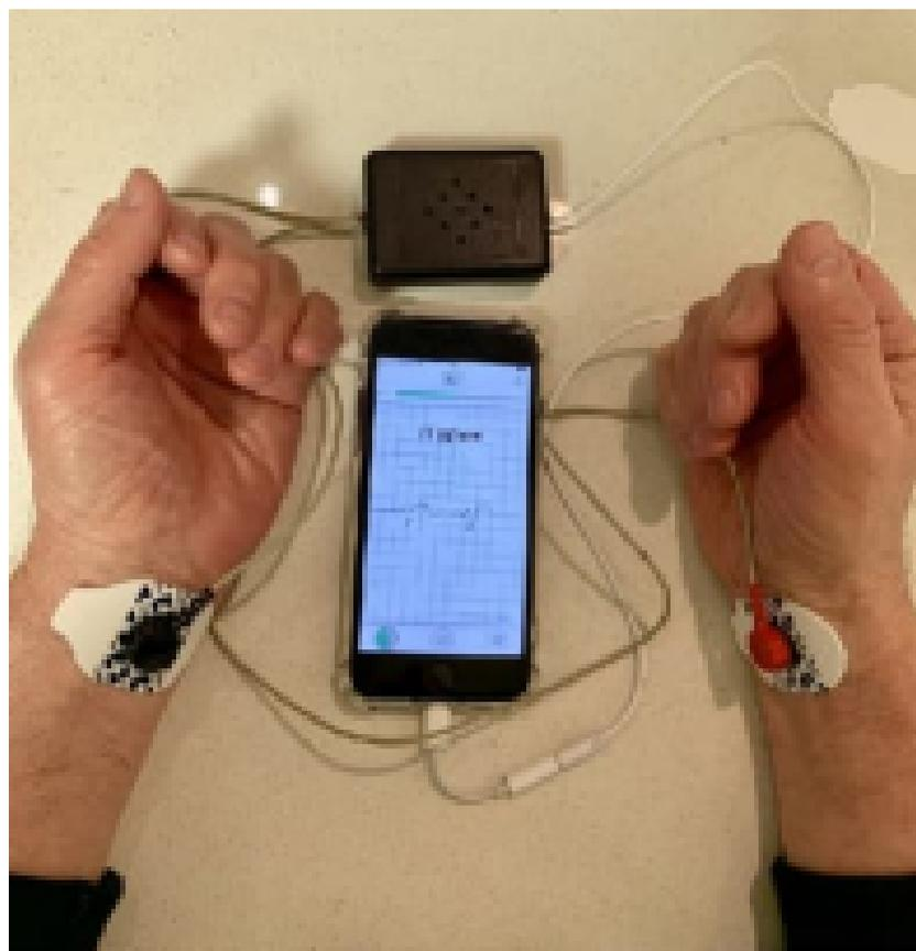
**Figure 6 — Connecting the ECG monitor.**
